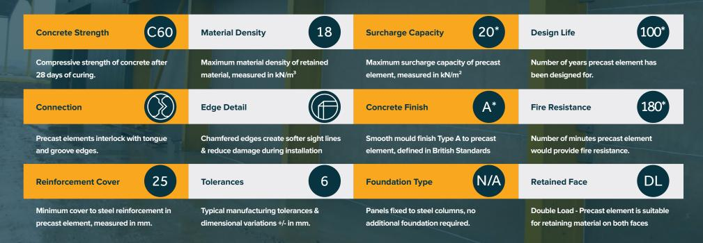
\* These are the maximum values that can be achieved with concrete panels, this will vary depending on the panel thickness & panel length. Concrete panel finish is class A to the front face and hand trowel finish to the back face.
